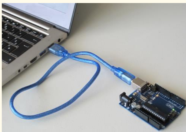
Figure 2 Connect your Arduino to the USB port of your computer. Source: www.getready.io/arduino
