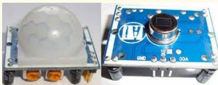
Figure 1 PIR Sensor, source: https://create.arduino.cc/projecthub/biharilifehacker/arduino-with-pir-motion-sensor-fd540a
