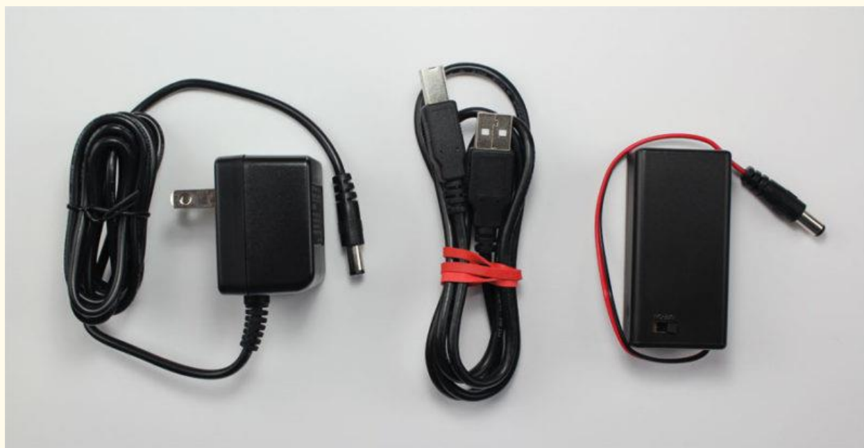
Figure 4 Arduino UNO power source, source: https://www.makerspaces.com/arduino-uno-tutorial-beginners/
