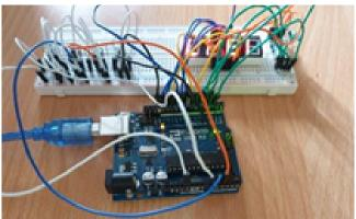
The students of the microcontroller course are working on a signal system (LED and tones) that will support compliance with the regular times for quick intense ventilation of the classroom (as part of the pandemic-related hygiene guidelines). This system will also be connected with a CO2 sensor and a thermal sensor to monitor the air quality and temperature in the classroom.
