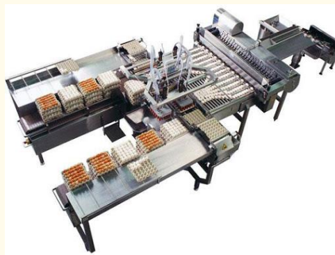
Figure 27 - Machine packing and weighing eggs (Ovobel, n.d.)
