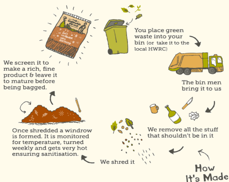
Figure 20 - Composting process (Greenaway, n.d.)
