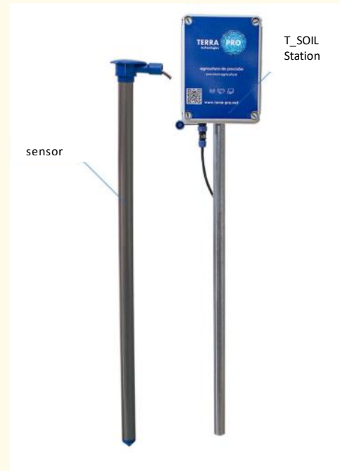
Figure 17 - T_Soil monitoring station (Agriterra, 2020)
